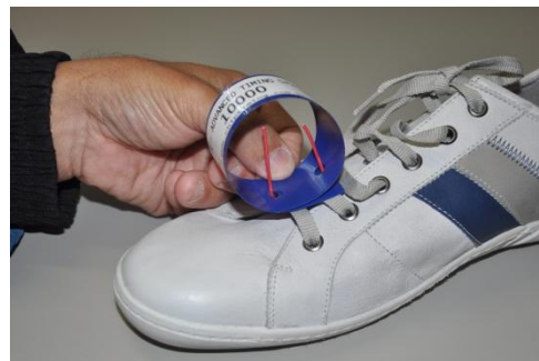
40. Introduce the wire through the both holes of the TAG and twist it around itself firmly.
